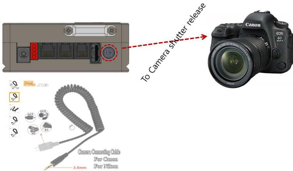
The shutter release cable that is connected to the camera can use the accessories of "Pixel TW-283 Shutter Release".
